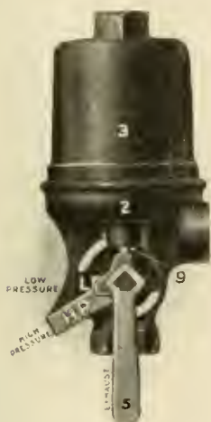
FIG. 3. HIGH AND LOW PRESSURE RETAINING VALVE.
